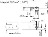
Example 1: Hinge clamps 1825011 Operating pressure 220 bar Standard clamping lever L = 22 mm
