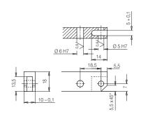
Example 1: Hinge clamps 1826011 Operating pressure 60 bar Standard clamping lever L = 22 mm
