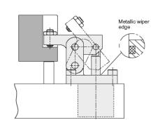
The mini hinge clamp is a low-cost hydraulic clamping element for thin-walled workpieces and reduced space.
