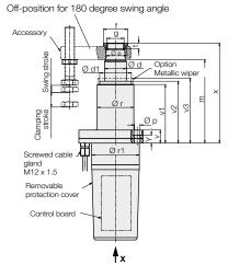
Collar nut included Option M Metallic in the delivery Spare nut see page 4 Ø d2 Clamping arms see page 4 Cable + cable plug Cable: 2x1.5mm 12x0,25mm2 as pe (Lapp Ölflex sturdy 210 black) Binder series 425 (79-6029-20-12) supply voltage shielded
