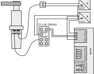
**IO-Link** connection Supply voltage 24 VDC -15A 1 +24 VDC
