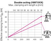
Example 2: 1885 102 single acting. For a desired effective clamping force  $F_{Sp}$  of 8 kN and use of a swing clamp 1885102 with a standard clamping strap 0354002 an operating pressure p of 345 bar is required.
