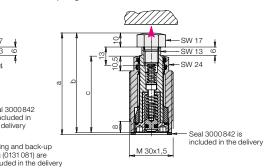
Adm. load [kN] 6.5 9.5 Stroke [mm] 8 8 а [mm] 80.5 90.5 b [mm] 79 89 [mm] 54.5 64.5 С Spring force min./max. 7/12 7/12 [N]
