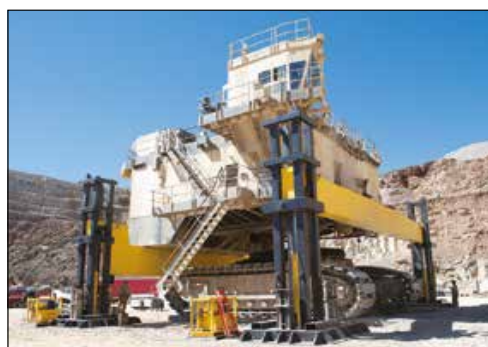
◀ A 1200-ton electric mining shovel being separated using custom 500-ton RR-Series cylinders and a pump per point synchronous lift system.
