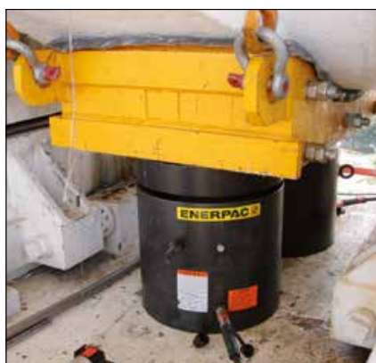
▲ Heavy lifting and foundation levelling. The lock nut provides mechanical load holding over a long period of time.
