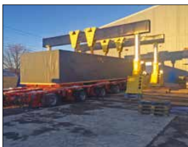
Hydraulic Boom Gantry Safely Transports 120 Ton Machine Bed
