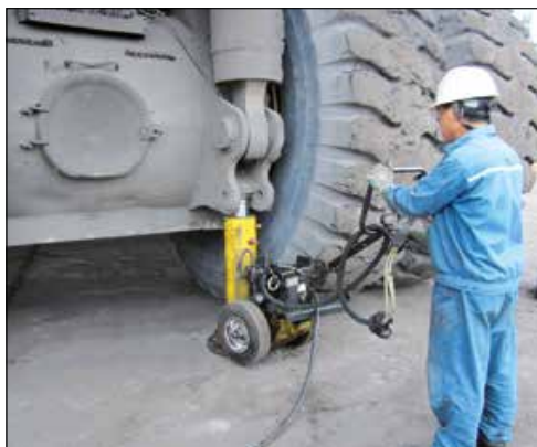
◀ Enerpac POW'R-RISER® used in mining operations to lift heavy equipment.
