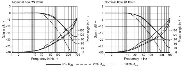
Dependence of frequency f at - 90 ° on working pressure p and input amplitude (measured with safety barrier <sup>1)</sup>)
