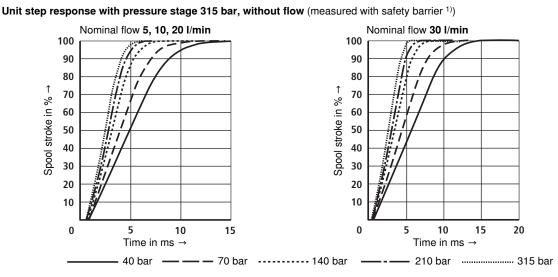
Frequency response with pressure stage 315 bar, stroke frequency response without flow (measured with safety barrier <sup>1)</sup>)
