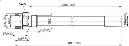
For version with long-distance line (E1, E3 or E5) and a length of 200 mm
