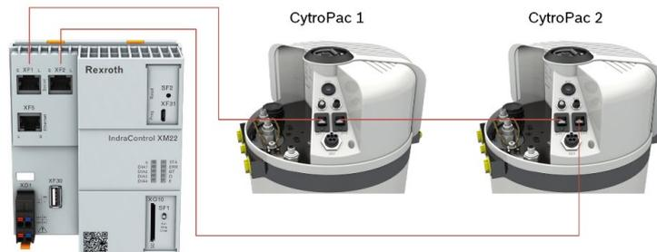
Abb. 54: Example of connection ring topology
