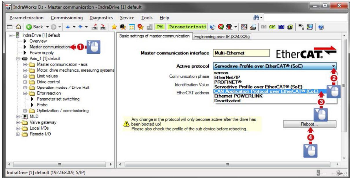
**Fig. 34: Activating EtherCAT® (CoE)**
