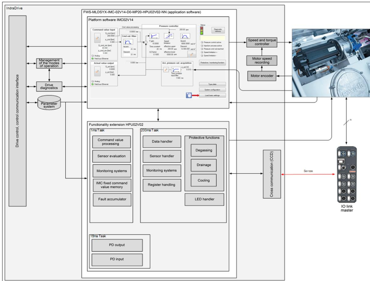
**Fig. 3: Structure of the application software**
