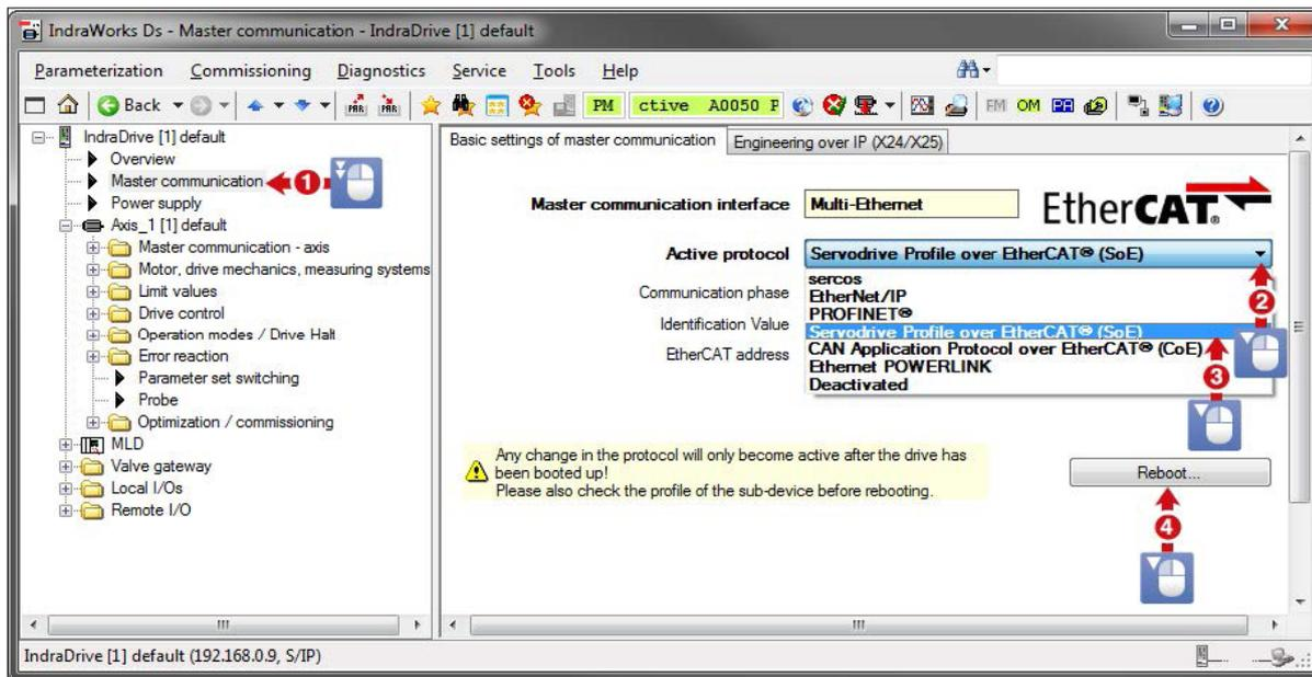
**Fig. 33: Activating EtherCAT® (SoE)**
