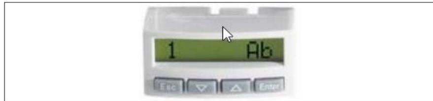
Fig. 1: Operating unit with 8-digit display (standard display)
