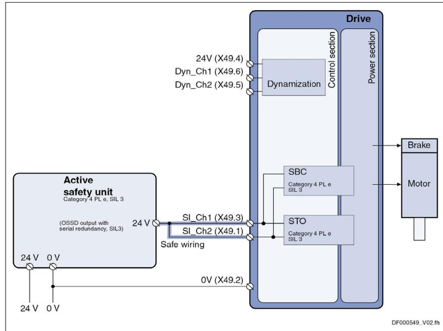
**Fig. 19: With active safety unit (plus-plus switching outputs)**
