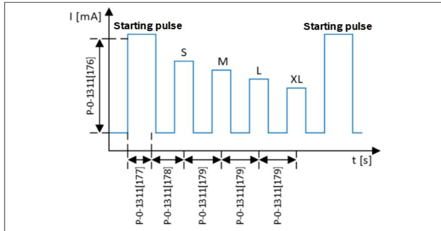
Fig. 4: Configuration of the evaluation of the serial signal of the particle sensor
