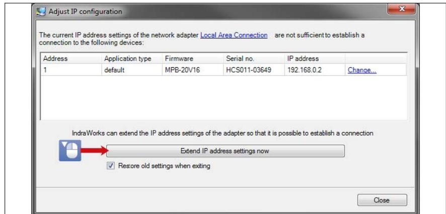
Fig. 25: Adding IP address settings
