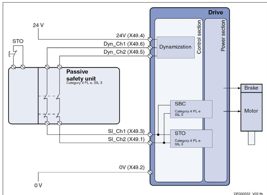
**Fig. 18: With two-channel wiring and passive safety unit**
