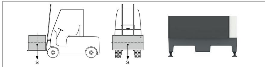
Fig. 11: Transport using a forklift
