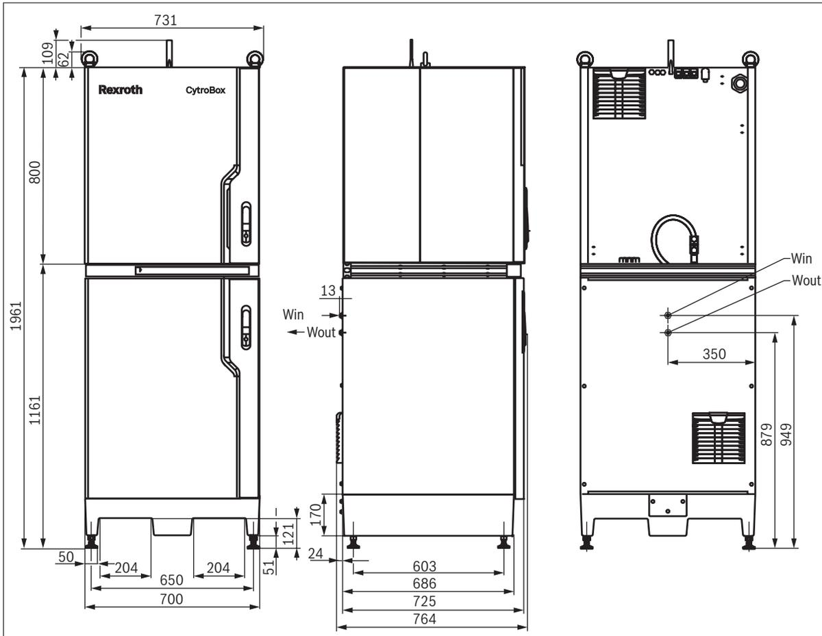
Fig. 13: Dimensions of the hydraulic power unit
