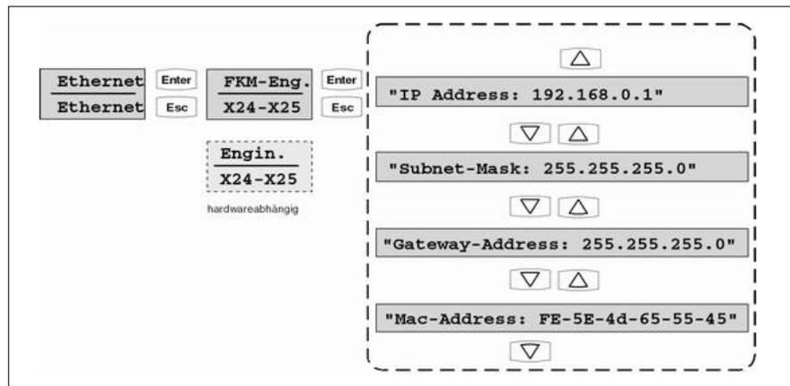
**Fig. 2: Example: Display of IP addresses**
