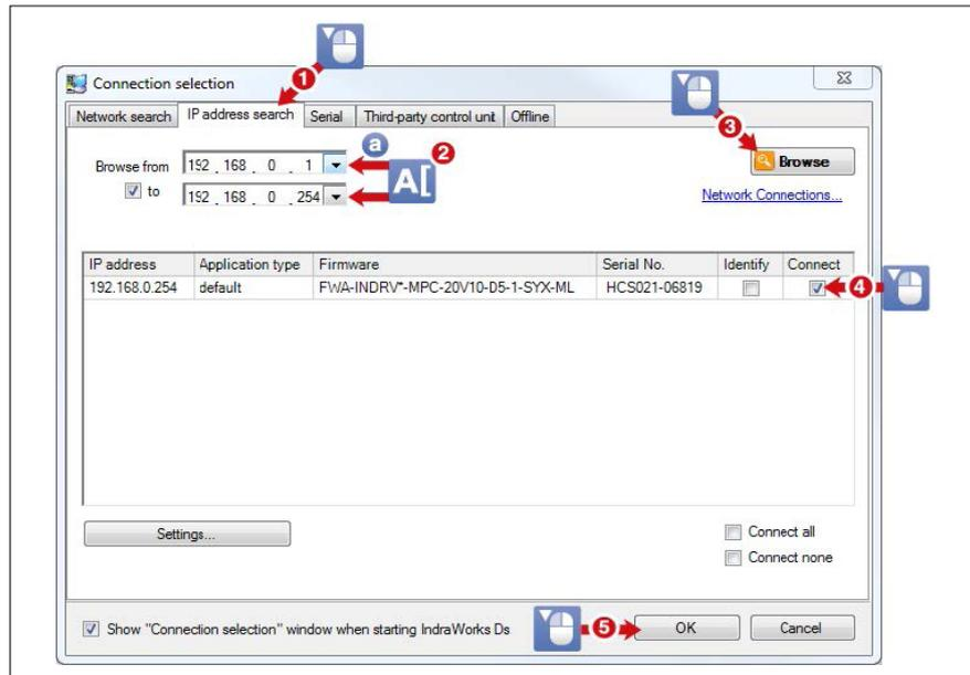
**Fig. 26: Establishing a TCP/IP connection to the drive via an Ethernet interface**
