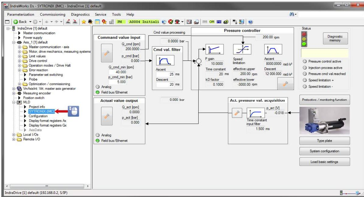
Fig. 36: Start dialog of the IMC software / parameter file
