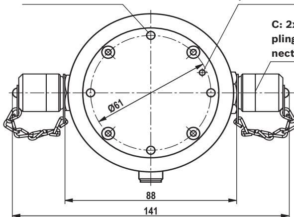
**B: Bleeding opening with pressure compensation element (fastened from the inside)**
