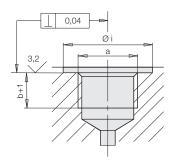
Sealing is attained by a knife edge at cylinder collar, requiring the sealing surface to be square to hole axis and flat.
