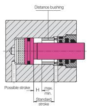
**Example: Possible stroke** Block cylinder 1545516 Standard stroke 50 mm
