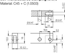
Example 1: Hinge clamps 1825011 Operating pressure 220 bar Standard clamping lever L = 22 mm
