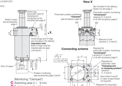
Switching area 2 ÷ 10 mm Use screws 12.9 Pneumatic valve Connecting holes: (actuated by the clamping arm) Silencer for pneumatic valve
