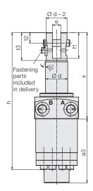
A = Clamping **B** = Unclamping
