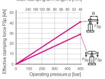
**Example:** 1895 106 An operating pressure p of 200 bar in connection with standard clamping arm 0354 003 of arm lenght L = 75 mm results in an effective clamping force FSp of 7 kN.
