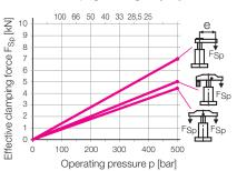
**Double acting (1895 X06)** Max. clamping arm length e [mm]
