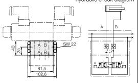
Presentation of twin non-return valve and twin flow control non-return valve
