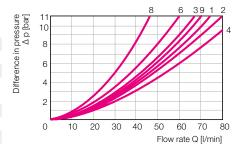
When determining pressure drop it should be noted that for double-acting cylinders with a piston surface ratio of e.g.  $\phi=1.6$  a return flow rate 1.6 times the flow rate of the power unit must be used.
