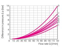
When determining pressure drop it should be noted that for double-acting cylinders with a piston surface ratio of e.g.  $\phi=1.6$  a return flow rate 1.6 times the flow rate of the power unit must be used.
