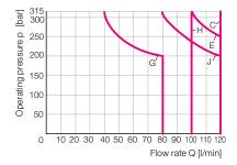
Note: The switching function of the valves depends on the filtering, due to the sticking effect. If the indicated, admissible flow values are to be used to the maximum, full flow filtering to 25  $\mu$ m is recommended. Besides this, the values are only valid for standard use with 2 flow directions, e.g. from P to A with simultaneous return flow from B to T.
