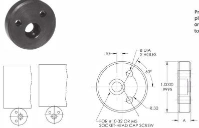
Precision side locator that can be doweled in place after adjustment. Use for vertical leveling or horizontal locating. Available hardened, or soft to allow drilling and reaming after installation.
