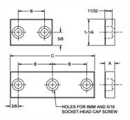
Large, precision rest pad for virtually any application. Peerless Rest Pads are extremely useful as supports, side locator pads, wear pads, or jig feet. Available both ground and unground for accurate height location. Mount with socket-head cap screws (not furnished).
