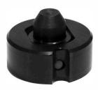
Provides precise location in one axis while allowing considerable float in the perpendicular axis. Use in conjunction with a Round Pin when loose workpiecehole tolerances require more float than a Diamond Pin would allow. Special pin diameters (A dimensions) are available. Please contact factory.
