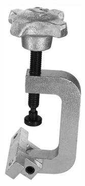
These unique C Clamps have a hinged pad for fastening permantently to a fixture, allowing them to swing clear for workpiece loading. The hinged mounting pad bolts to the fixture with two Socket-Head Cap Screws. Four-Prong Knob provides a firm grip for applications requiring quick tightening and high torque. Clamping screw is cast securely in the knob and has a removable swivel foot. Available in four sizes.
