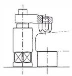
Swivel Contact Bolts are ideal for evenly distributing clamping pressure on sloped surfaces.
