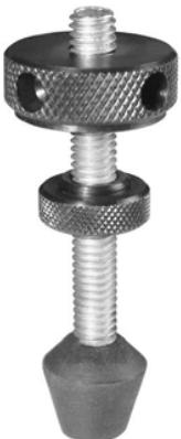
Same as the Flat-Cushion Spindles above, except with two knurled nuts, instead of hex jam nuts, for convenient hand tightening. Use for quick spindle adjustment in applications where high-torque tightening with a wrench is not required.
