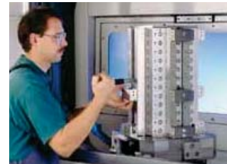
3. The clamping module is fixed by means of the eccentric screw and the torque wrench.
