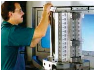
1. The clamping module with released eccentric locking is inserted in the high-precision slot.
