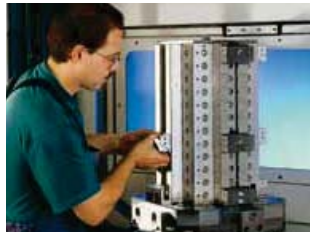
2. The clamping module is exactly positioned on the base module using the graduation marks and the scale.
