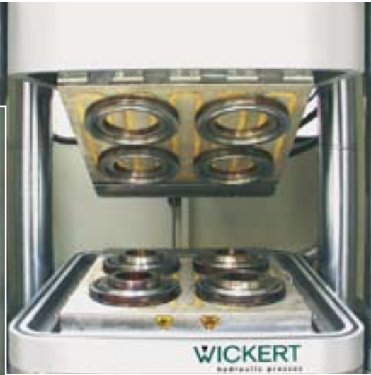
M-TECS 210 on a vertical press – various shapes on a machine bed without loss of space due to clamping claws
