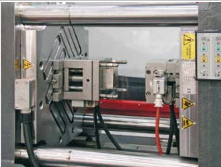
Even the smallest dies are securely held. Due to the long pole concentration effect maximum magnetic forces are transmitted into the die base plate. Machine FM 110 Electra, magnetic force 8 tons
