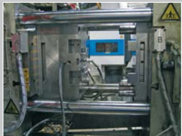
Magnetic clamping system on URPE diecasting machine CC 125, closing force 1500 kN, magnetic force 110 kN, temperature range 230° C
