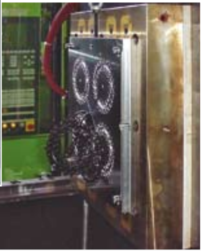
M-TECS 210 magnetic heating plate on an elastomer machine – full-surface magnetic force gives full-surface contact and more homogeneous temperatures.
