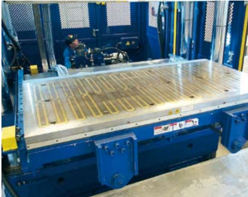
Magnetic clamping system on a vertical press for temperatures up to 240 °C
