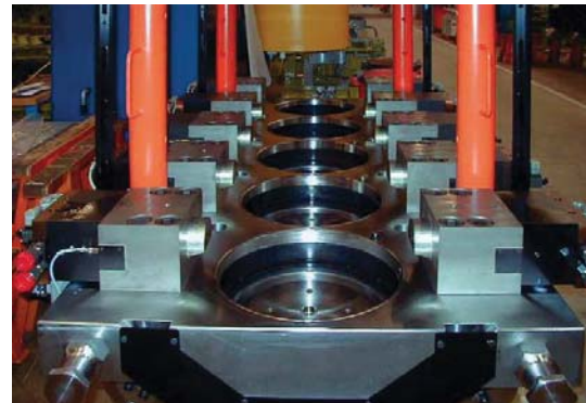
5-stage drop forging press equipped with wedge clamps with directional seat valves to activate the different stages
