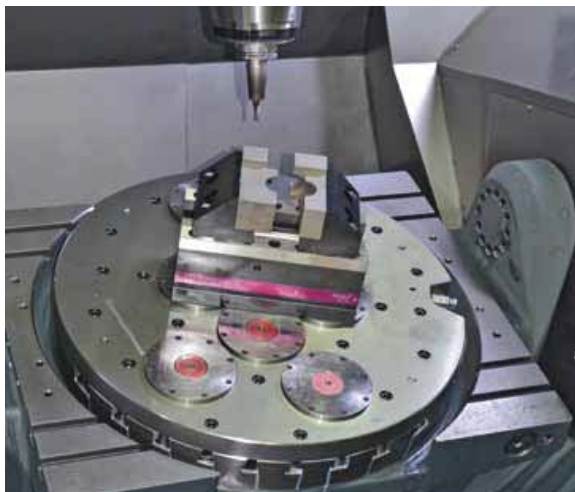
Workholding system MC 125 with workpiece-specific base jaw and form jaw used on a 5-axis machining centre.
