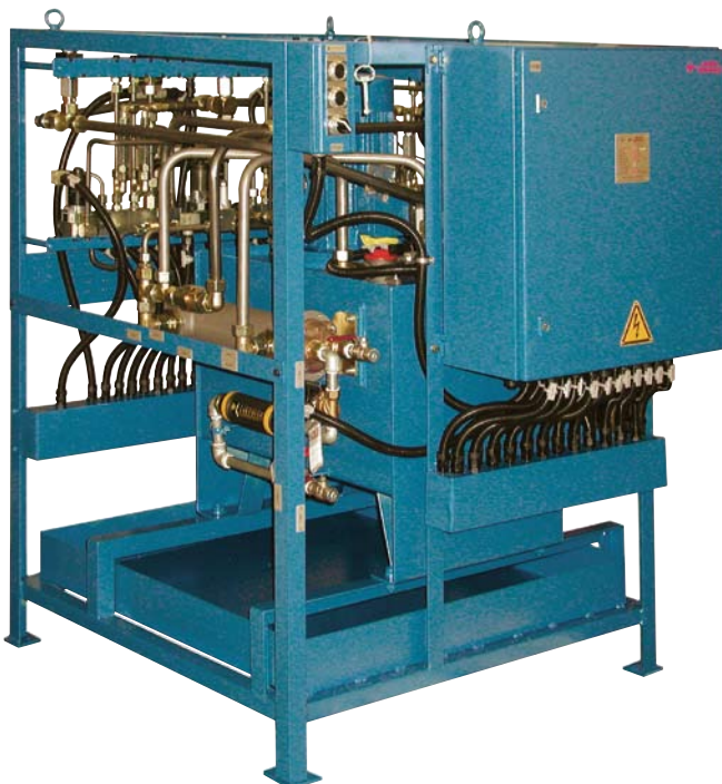
Frame-type power unit for 3 forging presses: 12 clamping circuits with pressure reduction for temperature compensation high pressure 4.2 l/min., 400 bar cooling return flow: 45 l/min., 10 bar
