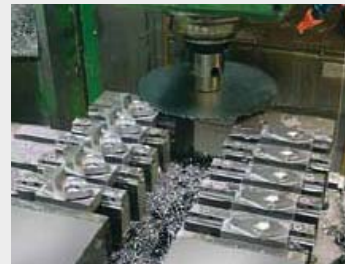
After finish-machining, the "lost head" is separated from the workpiece using a disk milling cutter.
