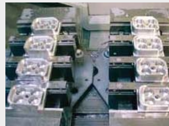
The clamping edge is milled off in the 2nd clamping step.
