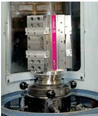
Tower workholding system TS 80 TriStar, a workholding system with connection to Maturra MAM 72
