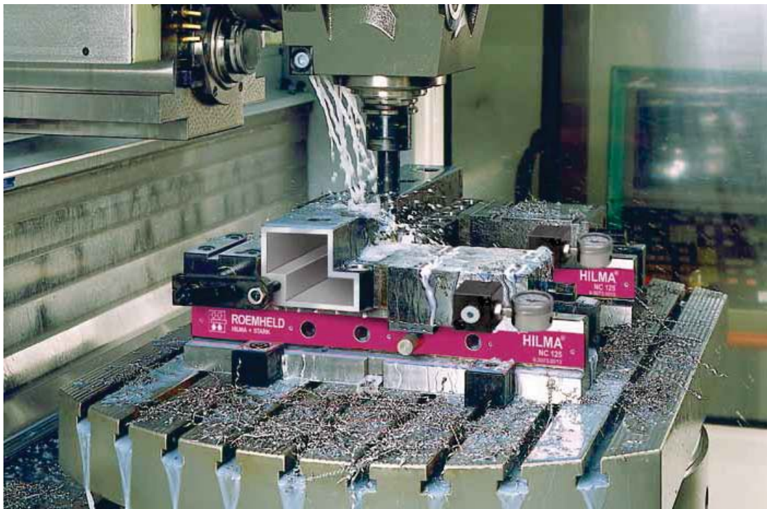
NC machine vice mechanical-hydraulic with clamping force display and top jaws
