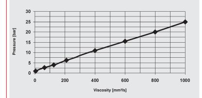
\* For a flow rate of 100 ml/min, flow control valve fully open, new filter element
