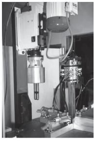
The figure shows the application of four station rotary indexing machine. In three operating stations the workpieces are bored by multiple spindle heads and threads are cut. At the load and unload station the machined workpieces are exchanged with unmachined ones. The pneumatic clamping elements are double-acting. The control is designed according to the circuit example on the next page; however every second port is not used.
