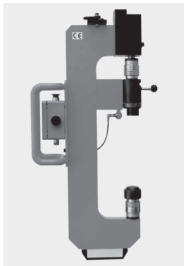
Mobile press-in frame for assembly, 25 kN version with mechanic pre-centring of the upper thrust bearing and electrical position monitoring. Application in the automotive industry: Assembly of front axles for utility vehicles.
