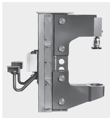
Mobile press-in frame for assembly, 80 kN version with opened lower thrust bearing for shafts. Application in the gear industry: Assembly of gears with one-part gear housings.
