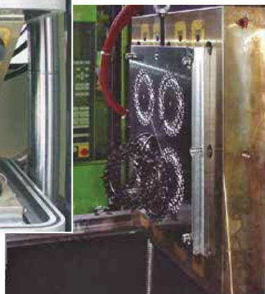
M-TECS 240 magnetic heating plate on an elastomer machine – full-surface magnetic force gives full-surface contact and more homogeneous temperatures
