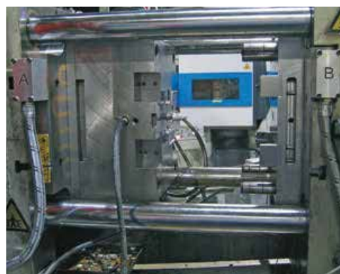
Magnetic clamping system on URPE die casting machine CC 125, closing force 1500 kN, magnetic force 110 kN, temperature range up to 240°C.
