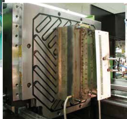
M-TECS 120 – An exceptional concentration of force: The magnetic force is transmitted through the long poles with double magnets into the clamping surface
