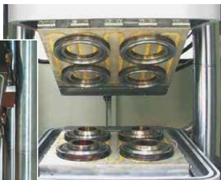
M-TECS 240 on a vertical press – various moulds on a machine bed without loss of space due to clamping claws
