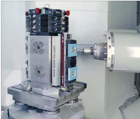
Clamping tower loaded with SPEEDY classic and couplings with blow off and integrated surface control systems
