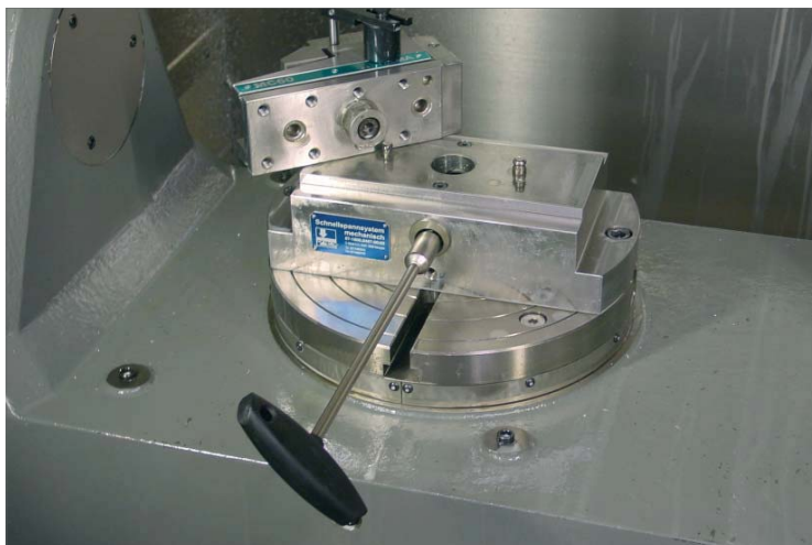
Fast clamping block with SPEEDY metec 2.
