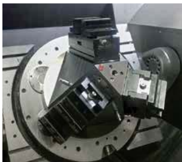
3 workholding systems MC-P in 3x120°-arrangement on a 5-axis machining centre.
