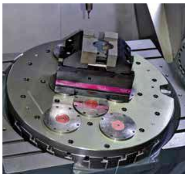
Workholding system MC-P Z with workpiece-specific base jaw and form jaw used on a 5-axis machining centre.
