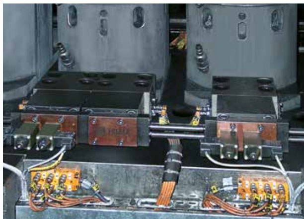
Wedge clamps with directly manifold-mounted directional control valves
