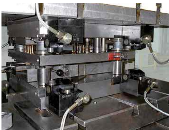
Angular clamp with T-slot adaptor in a high-speed punching press, the clamping force per clamping point is 66 kN
