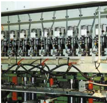
Electro-mechanical swivel and pull clamps mounted on a double-column press.
