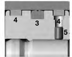
3. Double acting piston seal 4. Wear bands 5. Piston threaded and sealed to piston rod with permanent adhesive and mechanically secured with a set screw.
