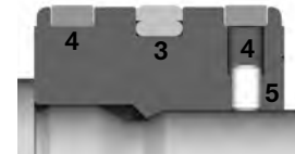
3. Low friction piston seal 4. Wear bands 5. Piston threaded and sealed to piston rod with permanent adhesive and mechanically secured with a set screw.
