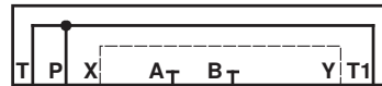
Fig. 68: Flushing plate according to ISO 4401-05-04-0-05 for valves NG10, representation of the internal ports
