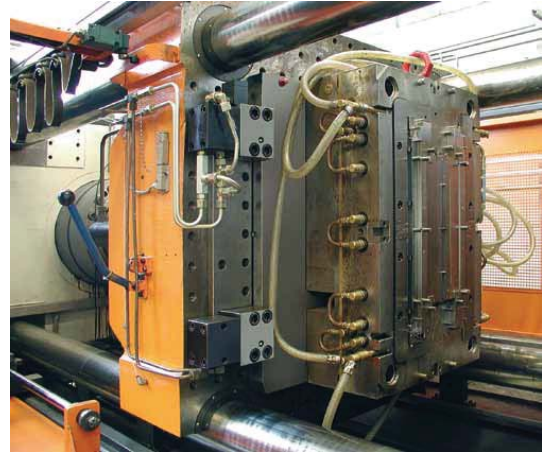
Wedge clamp with check valve on a Krauss Maffei KM 575 injection moulding machine
