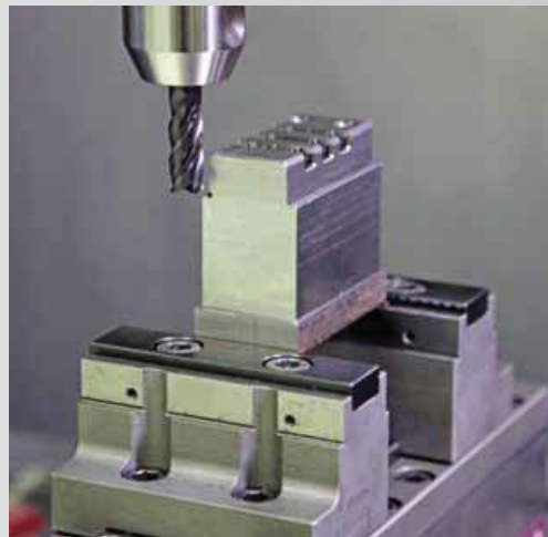
Grip jaw with steps for first and second clamping
